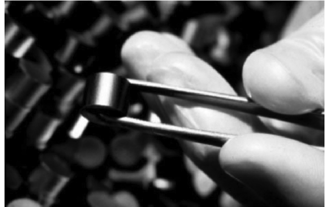
Figure 26.4 \text{UO}_2 pellet. (U.S. Nuclear Regulatory Commission.)
