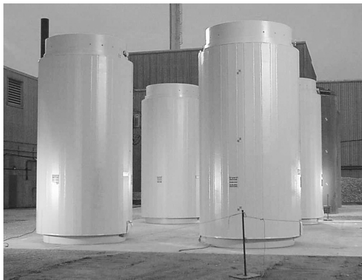
Figure 16.2 Dry storage casks for spent nuclear fuel. Source: Holtec International, http://www.holtecinternational.com/ .
