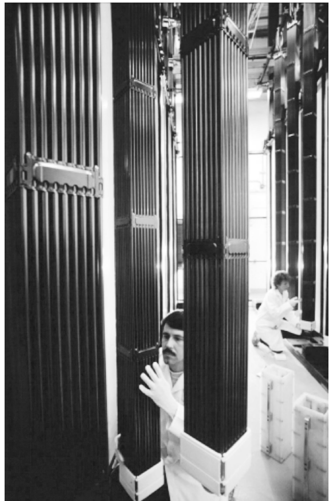
Figure 26.5 LWR fuel assembly. (U.S. Nuclear Regulatory Commission.)
