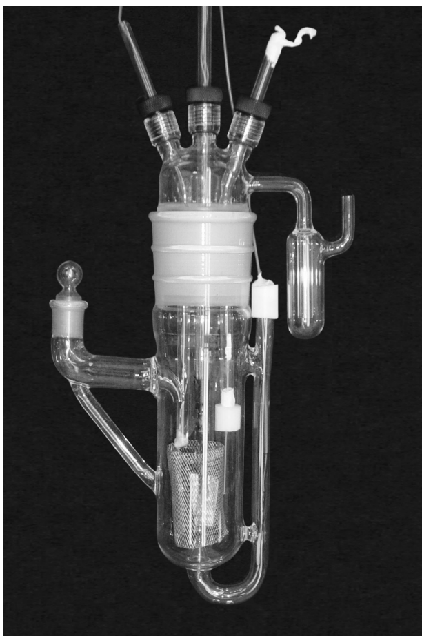
Figure 41.16 1990 SPAWAR first-generation cold fusion co-deposition cell (Courtesy of S.B. Krivit).
